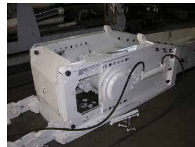
Return station with adjustable chain tension
